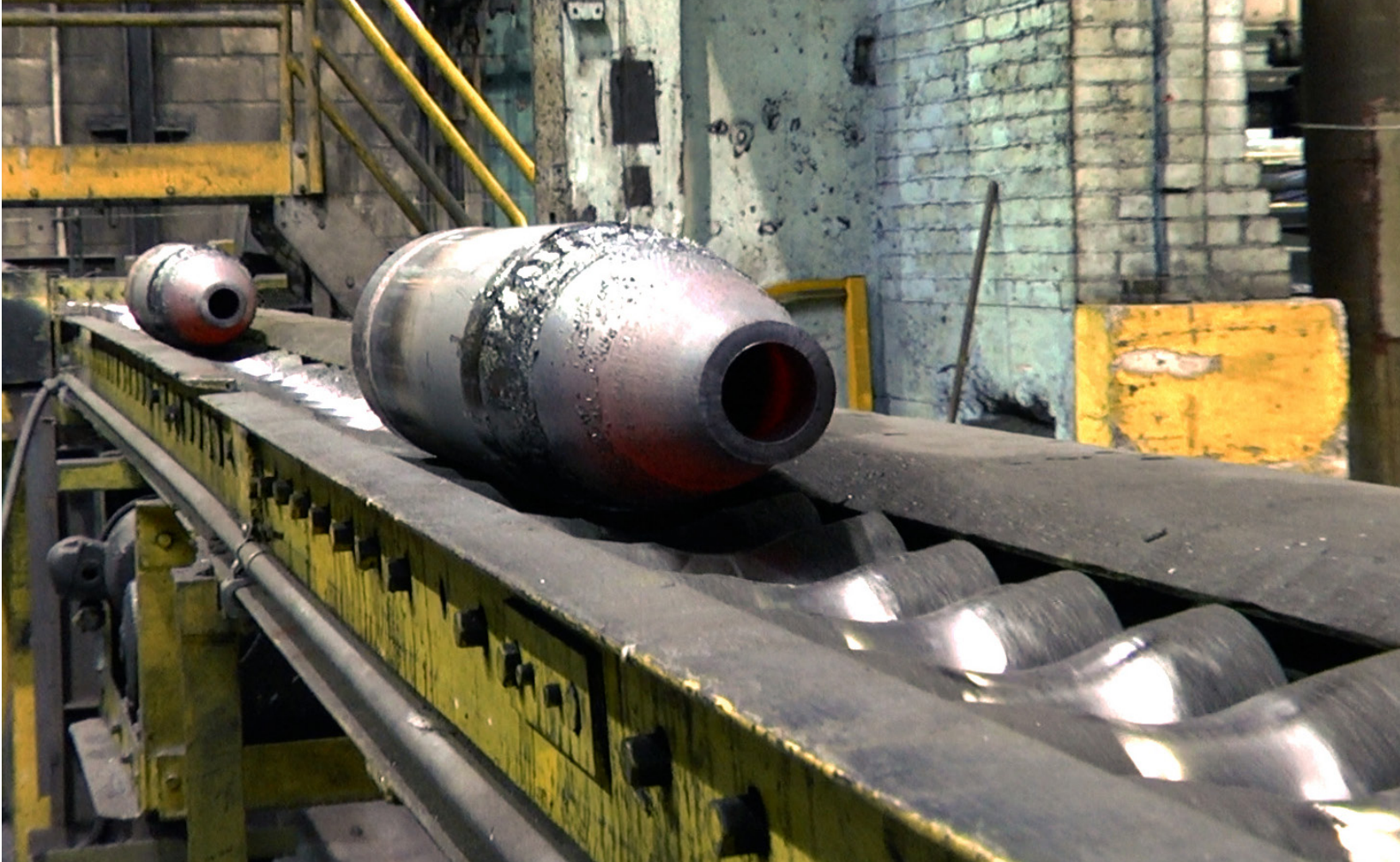
Scranton Army Ammunition Plant's nosing process is depicted as ammunition parts move on a conveyor to the heat-treating process. Credit: Dori Whipple / US Army Joint Munitions Command
